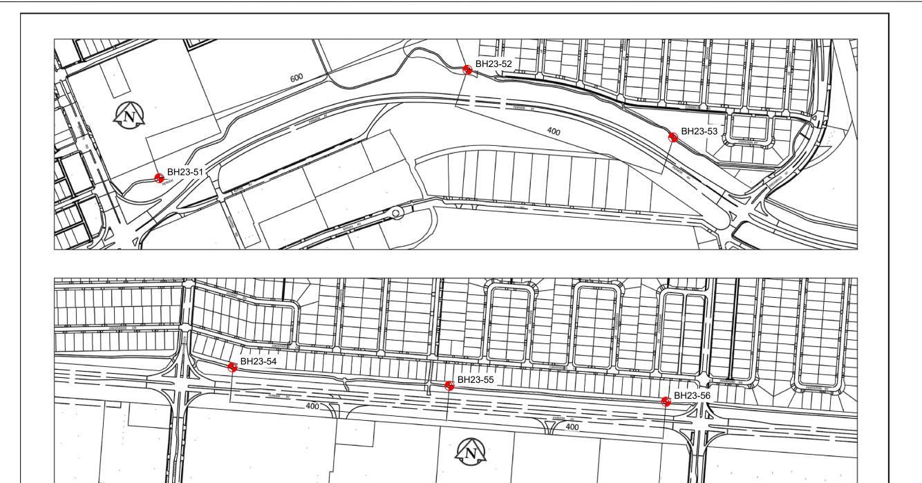
NOTE: -GEOTECHNICAL TESTHOLES 1m DEPTH -PATHWAY RECONSTRUCTION
